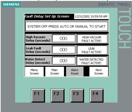
If you have special circumstances that require you to *delay the alarms from going off* then continue with this step, if not skip forward. <u>All of the alarm descriptions will show up on the right hand window as shown, and also on the Main Operations Screen.</u>
