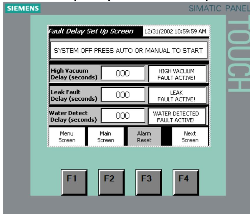
If you have special circumstances that require you to ***delay the alarms from going off*** then continue with this step, if not skip forward. **All of the alarm descriptions will show up on the right hand window as shown, and also on the Main Operations Screen.**
